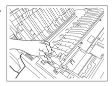
**5** Lift the original feeding tray and remove any misfed originals.
